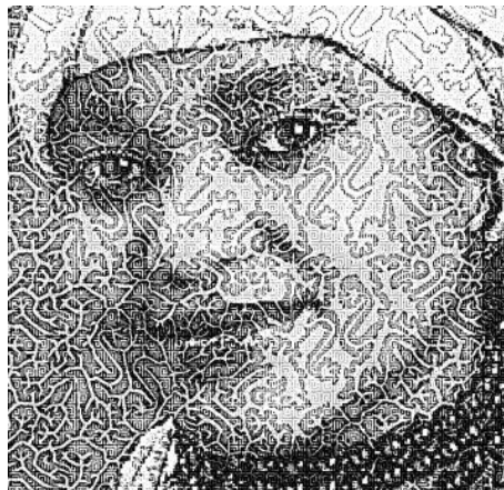
Girl image formed by a dragon microstructure and a greek frieze nanostructure.
